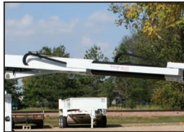
■ Hydraulic hoses supported with high strength hose track.
