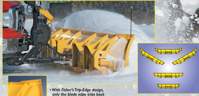
only the blade edge trips back when an obstacle is encountered. Since the blade and wings stay upright, you don't lose the load.
